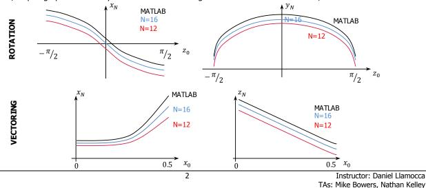
• Compute the MSE for each case. This metric assesses how close the hardware results are to the ideal ones (function values to which the CORDIC results converge). The smaller the MSE, the more accurate the hardware results are.
